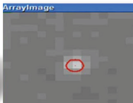
Fig.38: FV300 location and size information on the IR array
