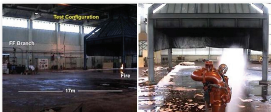
Fig.39: Test fire and extinguishment monitor in action
