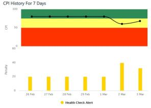
Trending of the CPI score provides information on how the chiller's performance is changing over time. When corrective actions are taken, an improvement in the CPI score can quickly validate that the root causes were fixed.
